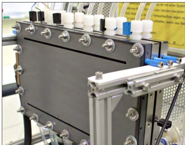
FIGURE 15. Flow electrochemical cell from Condias. Source: Photo from the authors.
