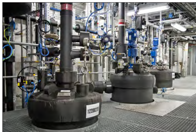
FIGURE 12. Pilot plant from Fraunhofer CBP (Leuna, Germany) to produce organosolv lignin. Source: Photo from the authors.
