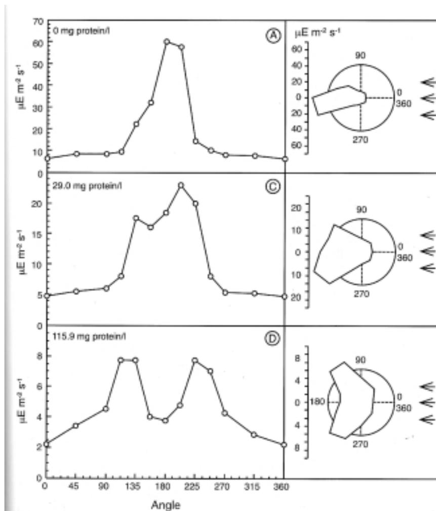
**Fig. 3** Irradiance as a function of the output angle in cultures of *Allochromatium vinosum* at different biomass concentrations. The results have been represented as X-Y graphs and polar plots. Arrows indicate the position of the light source
