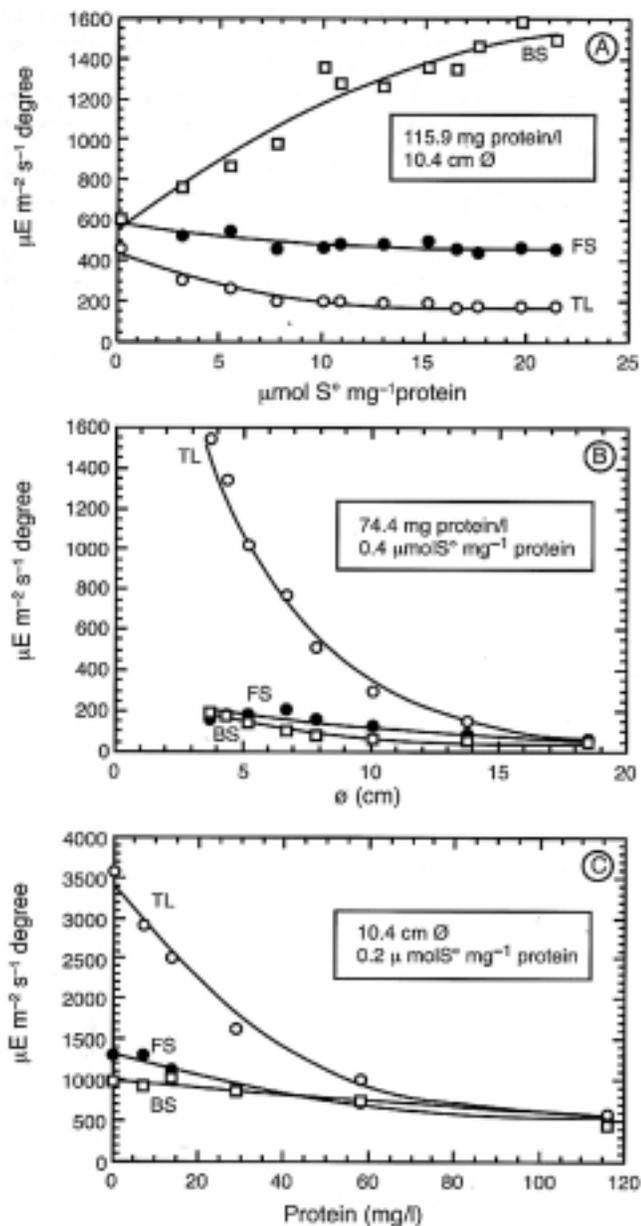
**Fig. 5** Amounts of transmitted (TL) (○), forward scattered (FS) (●) and backward scattered (BS) (□) light output as a function of: (A) the specific content of sulfur, (B) the diameter of the culture vessel and (C) the protein concentration. The conditions for each set of experiments are specified in the plots
