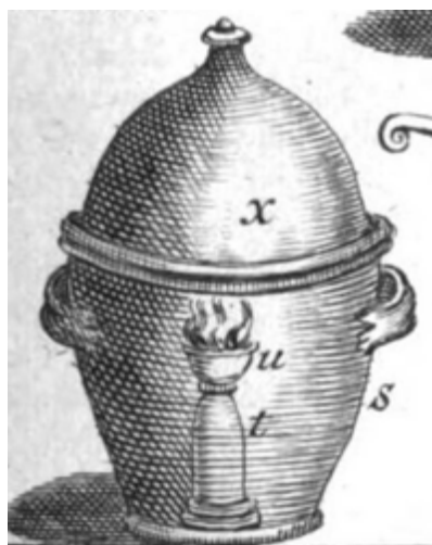
Figure 3. A device used by Nicolas Lemery for the production of sulphuric acid per campanam .
