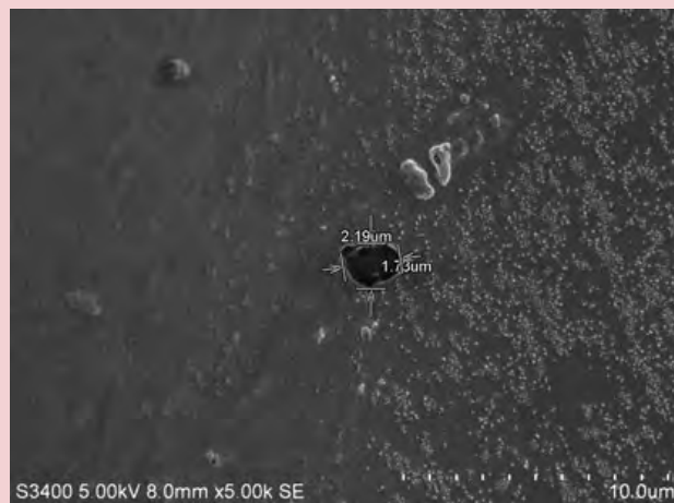
Figure 7. SEM image of cling film \times 5.00 keV.
