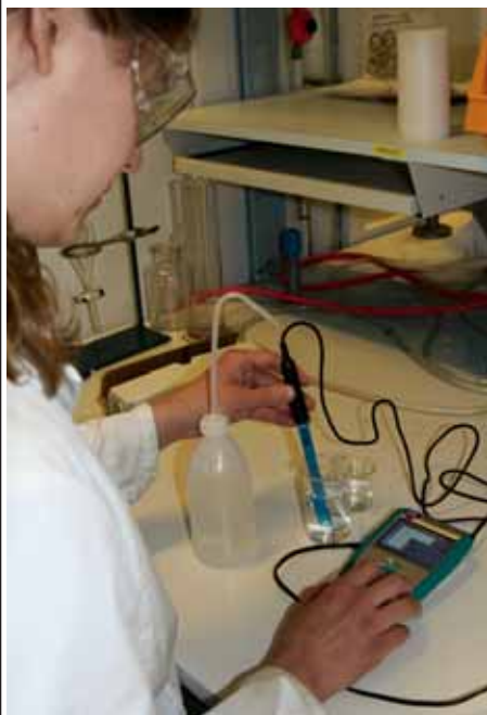
Figure 5. A student performing a pH curve registration and the corresponding graphic.
