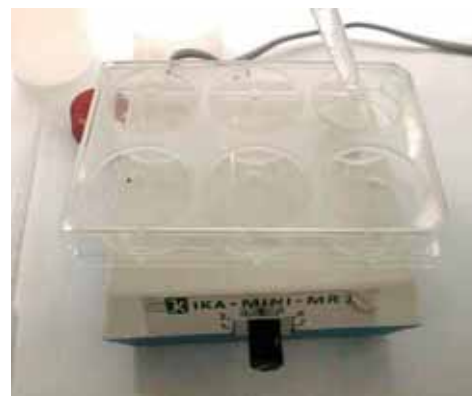
Figure 4. Green chemistry approach. A plastic microscale template used as a calorimeter.
