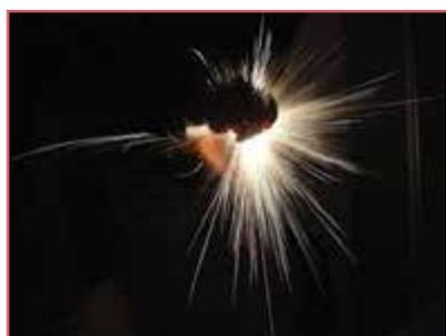
Figure 15. Sparks when the balls collide with aluminium foil in between.
