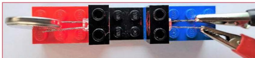
Figure 6. Juxtaposition of an emitting and a receiving LED with a LEGO construction.
