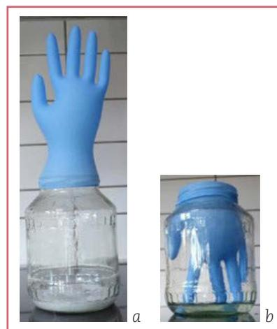
Figure 3. Expanding glove (a) against the air pressure and inverted glove (b) driven by the air pressure.
