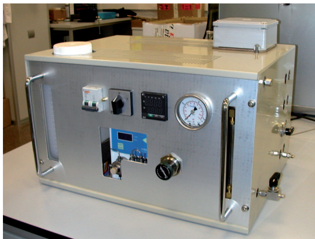
Fig. 5. Bio-ethanol reformer equipped with catalytic monoliths and a separation membrane selective to hydrogen. The permeate is hydrogen of high purity that can be feed directly into a low-temperature fuel cell for mobile applications.
