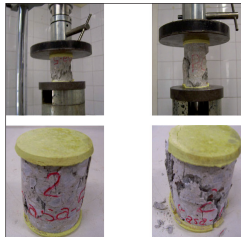
Figure 4. Compressive strength of the PCM-concrete.
