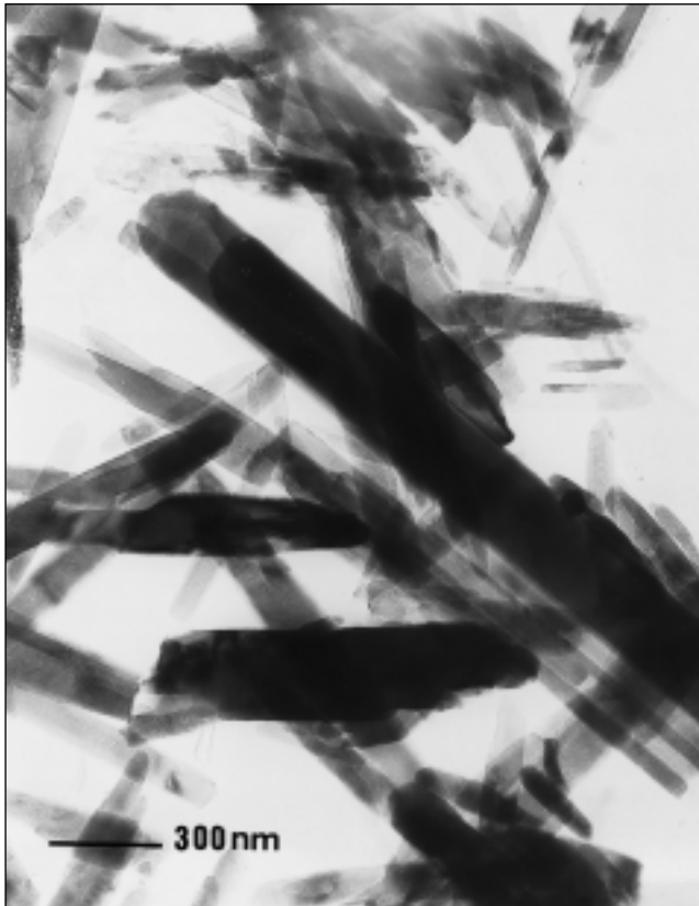
Figure 13. Transmission electron micrograph of hydroxyapatite obtained in a MSMPR reactor.
