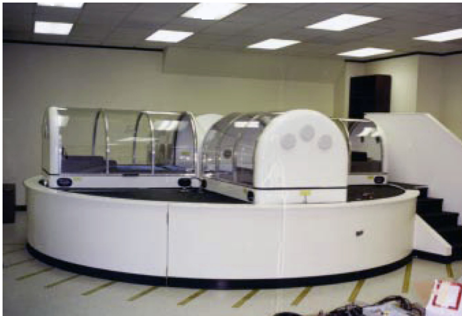
Fig. 2. Rotating platform used both in spacecraft, to reproduce gravity, and on Earth, to study the effects of greater or lesser gravitational forces on human biological functions.
