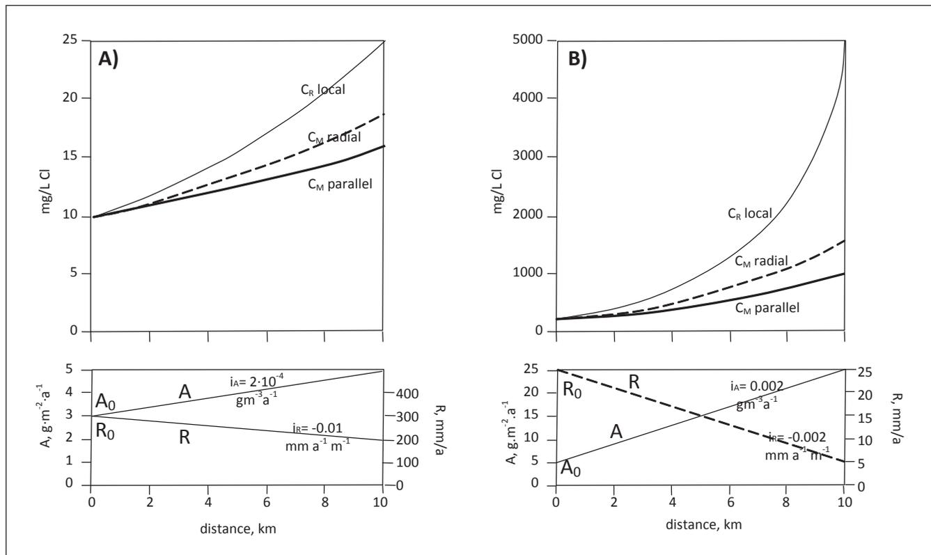
**Fig. 2.** Recharge in a sloping aquifer, showing chloride concentration in local recharge and the average value through the aquifer thickness, at increasing distance from the upslope boundary or apex in parallel flow and radial flow, respectively. **(A)** Well-recharged aquifer (humid climate) with slightly changing, moderate chloride deposition. **(B)** Poorly recharged aquifer (arid climate) with changing chloride deposition (proximity to the coast).
