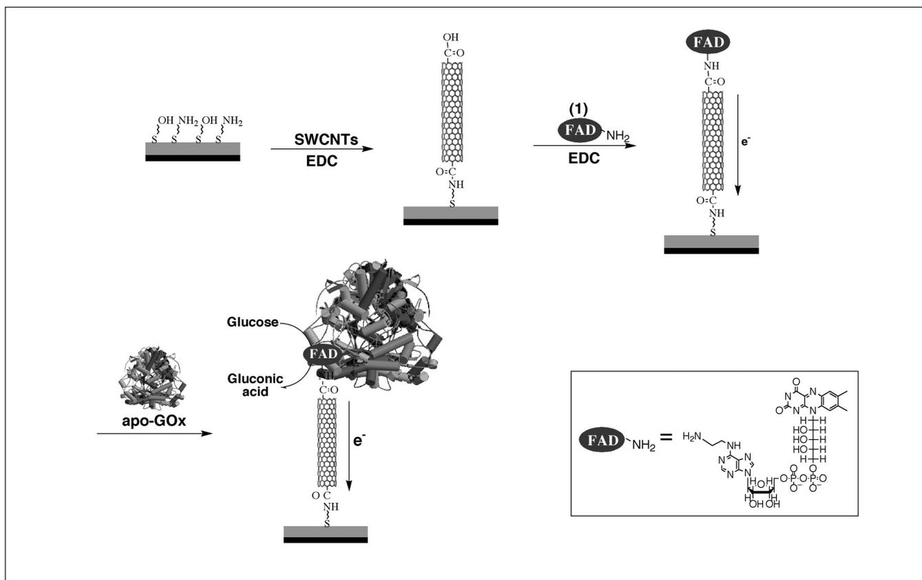
Figure 3. Assembly of the glucose oxidase-reconstituted CNT bioelectrocatalytic electrode.
