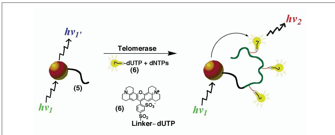
Figure 5. Optical detection of telomerase activity by the use of semiconductor quantum dots.
