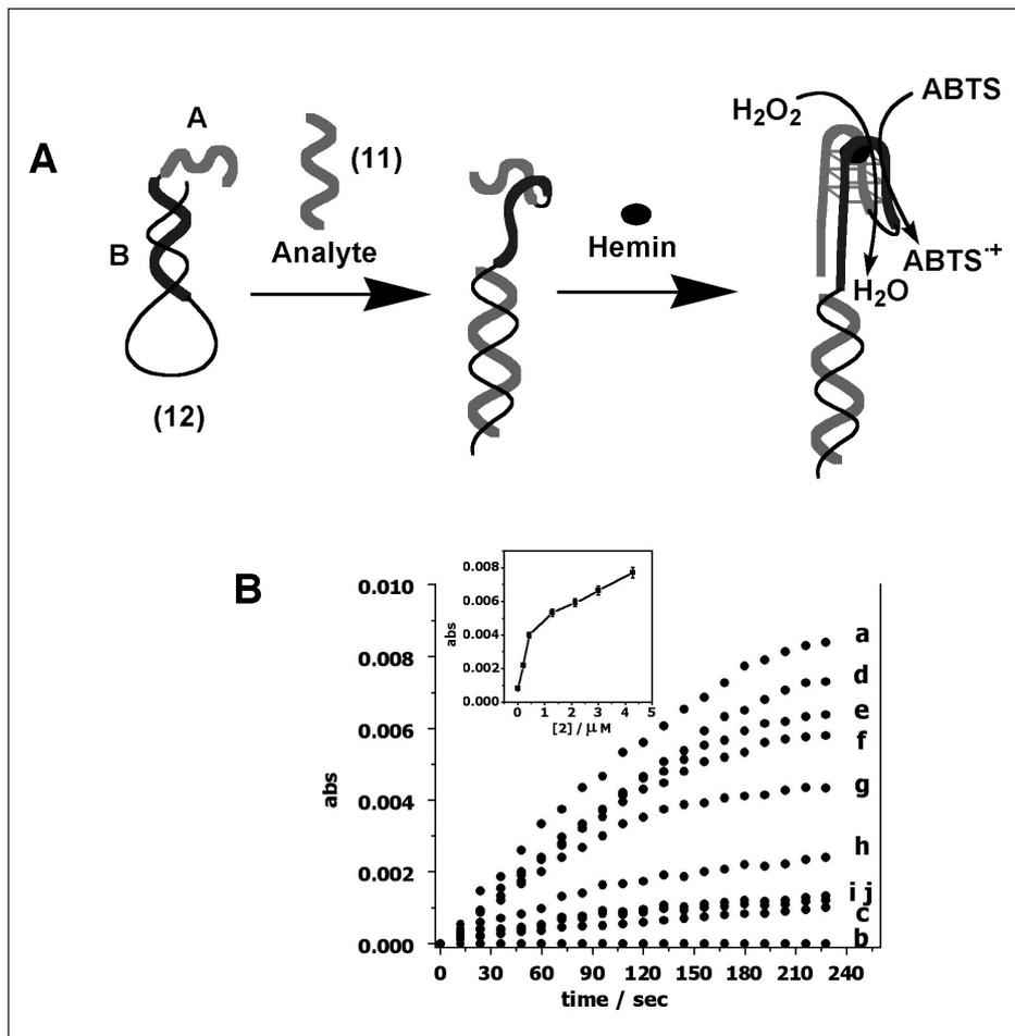
Figure 9. (A) Analysis of telomerase activity by a functional DNAzyme beacon system. (B) Absorbance changes as a result of the oxidation of ABTS upon analyzing the DNA (11) with the catalytic beacon (12): (a) 4.3 μM of (11); (b) in the absence of (11); (c) in the presence of (11) and hemin, but without (12); (d) to (h) in the presence of 3.0, 2.15, 1.30, 0.40 and 0.20 M of (11); (i) and (j) analyzing single base mismatches of (11), 4.3 μM.
