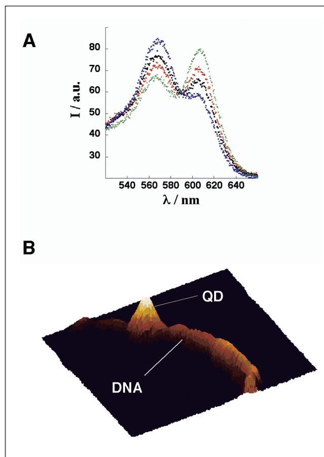
Figure 6. (A) Fluorescence spectra of the (5)-functionalized CdSe-ZnS quantum dots upon telomerization of (5) in the presence of HeLa cells extract (10,000 cells) in the presence of dNTP and (6) for different time intervals: before addition of telomerase; and after 10, 30 and 60 minutes; in the presence of telomerase before the addition of dNTPs and Texas Red-dUTP. (B) AFM image of the CdSe/ZnS-telomer conjugate.
