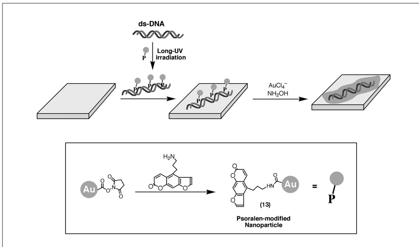
Figure 10. Assembly of a Au NP wire on a DNA template.
