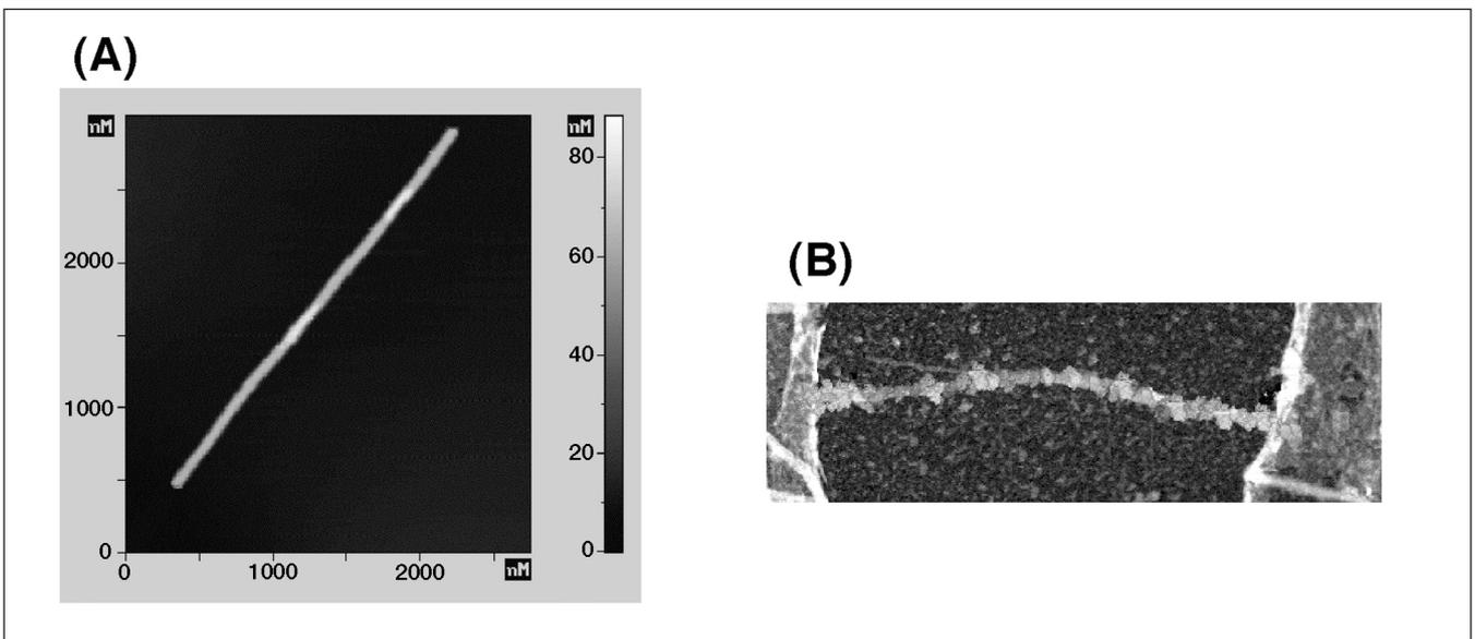
Figure 13. (A) AFM image of Au-nanowire on the actin template. (B) SEM image of the Au-nanowire on the actin template that bridges and contacts two Au microelectrodes.
