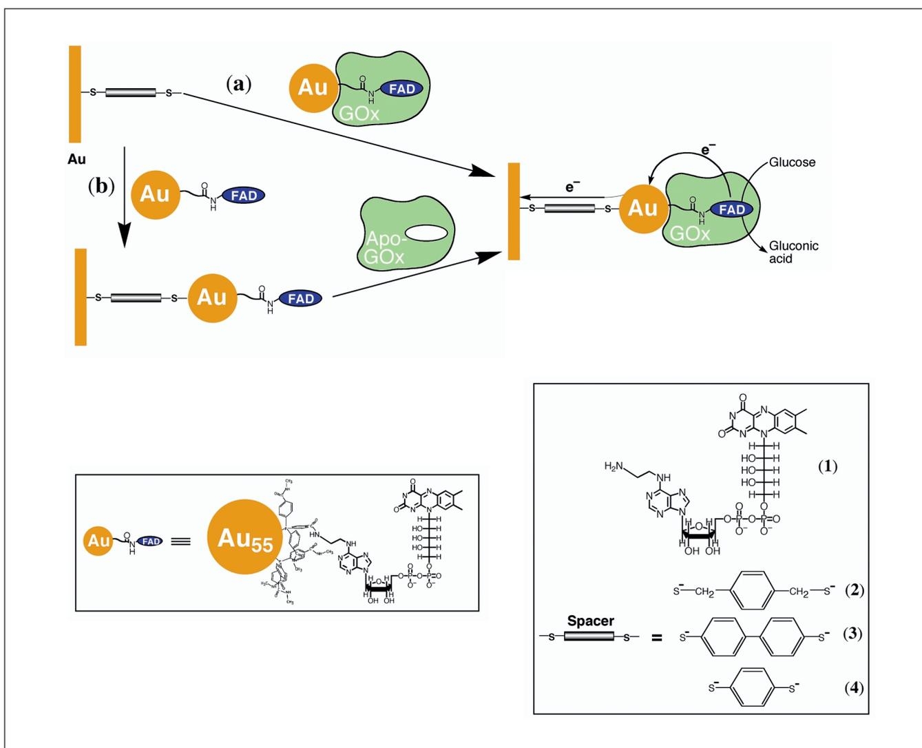
Figure 1. Electrical contacting of GOx by the assembly of GOx reconstituted on a Au-NP associated with a Au-electrode for the bioelectrocatalyzed oxidation of glucose.
