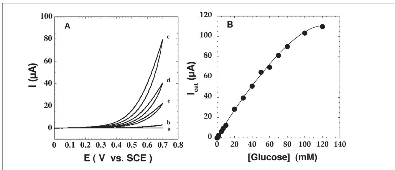
Figure 2. (A) Cyclic voltammograms corresponding to the bioelectrocatalyzed oxidation of different concentrations of glucose by the GOx-Au-NP-modified electrode. Glucose concentrations correspond to: (a) 0 mM, (b) 1 mM, (c) 10 mM, (d) 20 mM, (e) 50 mM. Data recorded in 0.1 M phosphate buffer, pH = 7, 35°C, scan rate 5 mV·s<sup>-1</sup>. (B) Calibration curve corresponding to the amperometric responses of the electrode at E = 0.6 V vs. SCE at variable concentrations of glucose.
