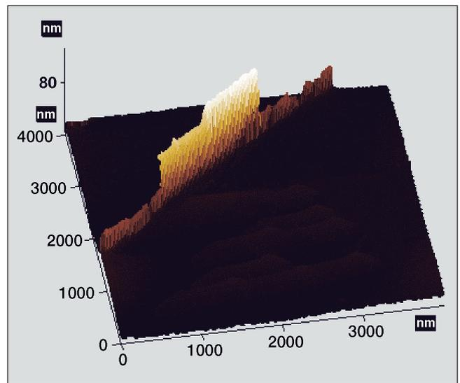
Figure 14. AFM image of the actin-Au nanowire-actin nanomotor.
