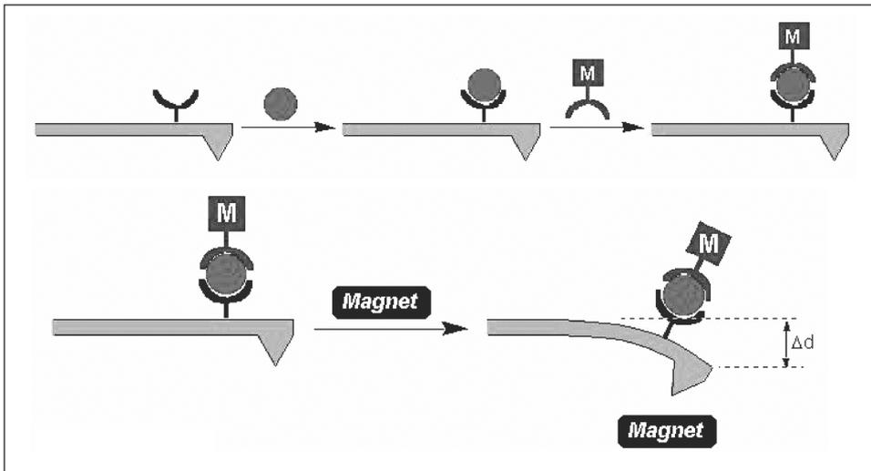
Figure 15. Amplified analysis of biorecognition events on a cantilever using functional magnetic particles and an external magnet.
