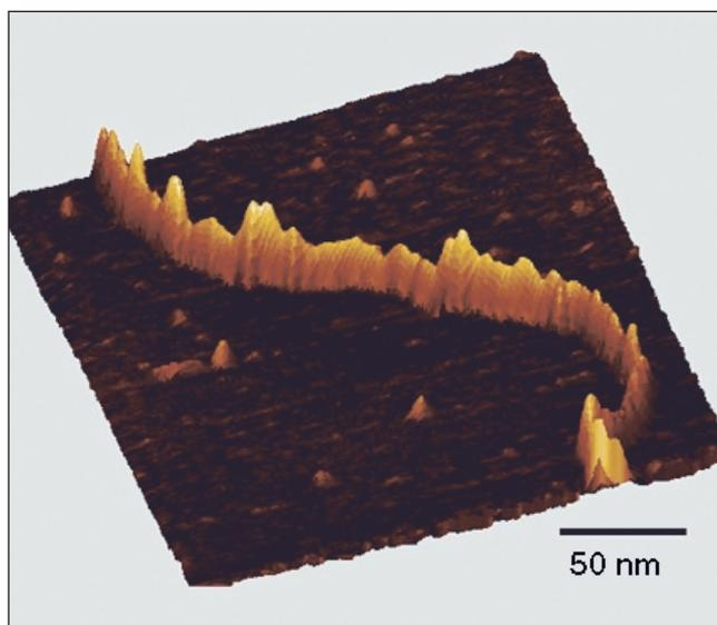
Figure 11. AFM image of psoralen-functionalized Au-NPs intercalated into polyA/poly T and photochemically crosslinked.
