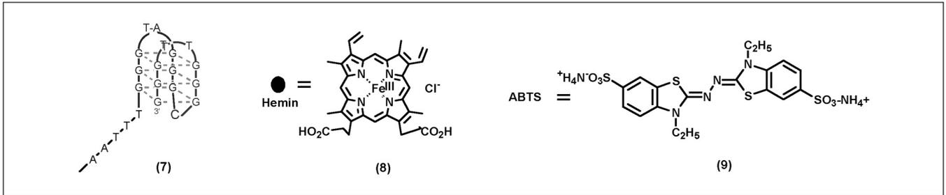
Figure 7. A hemin/G-quadruplex that catalyzes the oxidation of ABTS or stimulates the generation of chemiluminescence.
