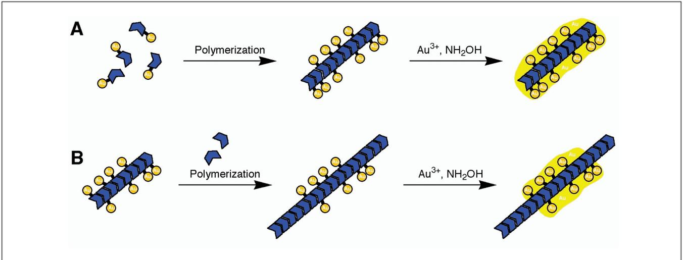
Figure 12. (A) The fabrication of a Au nanowire on an actin template. (B) The synthesis of an actin-Au-nanowire-actin hybrid system.
