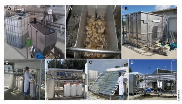
Fig. 3. (A) Pilot-scale moving bed biofilm reactor, (B) pilot-scale membrane bioreactor, (C) solar-driven pilot-scale photocatalytic reactors, (D) ultrafiltration pilot unit.
