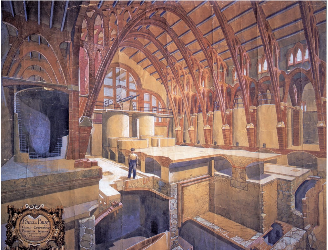
FIGURE 7. El Pinell de Brai. Winery of the Sindicat Agrícola. View of the interior with a structure of balanced arches. 1918.
